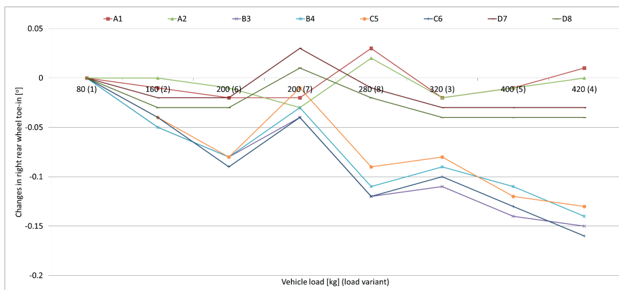
Figure 15 Dependency of changes in the right rear wheel toe-in on the weight distribution
