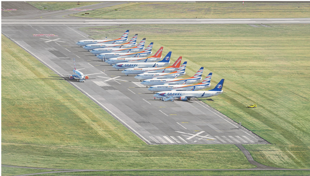
Figure 1 Closed RWY 04/22 at Praha/Ruzyně airport with COVID-19 grounded aircraft parking; marked with 'closed runway marking'; author: Vocolka, T.
