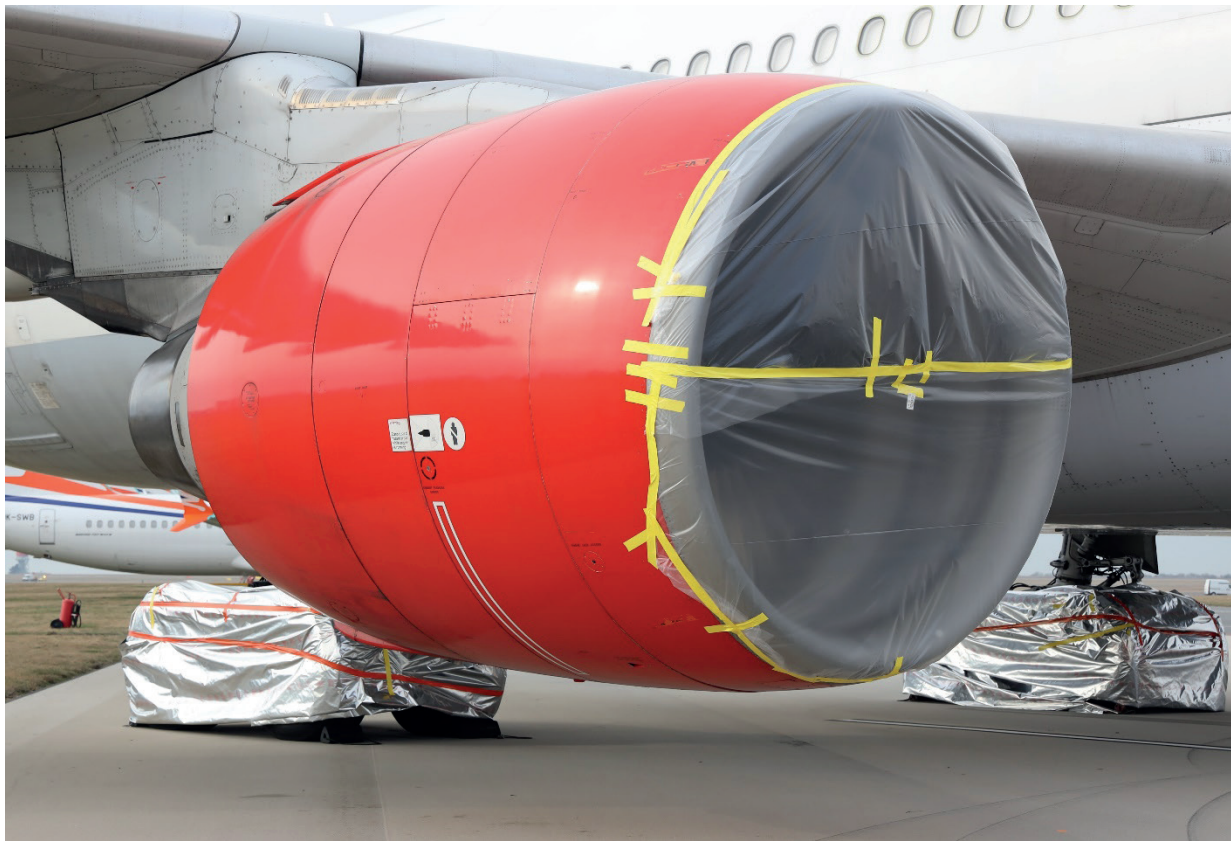
Figure 4 Engine inlets properly sealed and wheels thoroughly covered; author: Melus, M.
