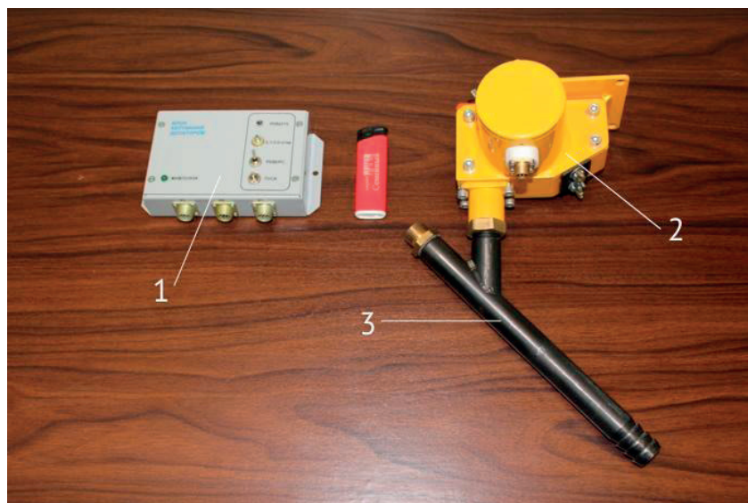
Figure 4 Sandbox design: 1 - control unit; 2 - sand supply dispenser; 3 - nozzle
