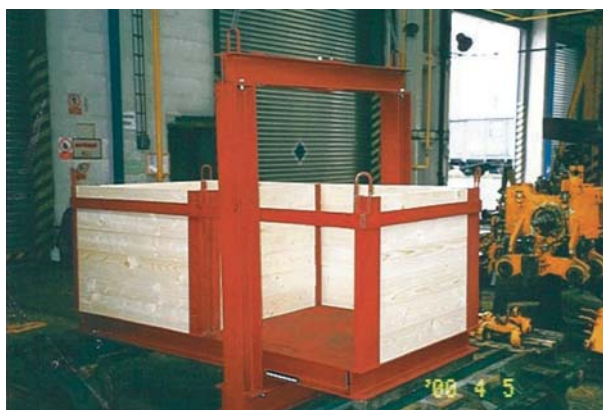
Fig. 1 View of testing box with inserted partition
