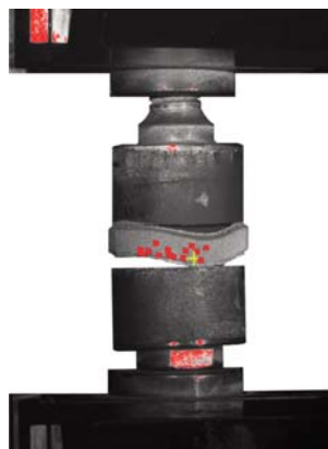
Fig. 3 Tearing of the test specimen
