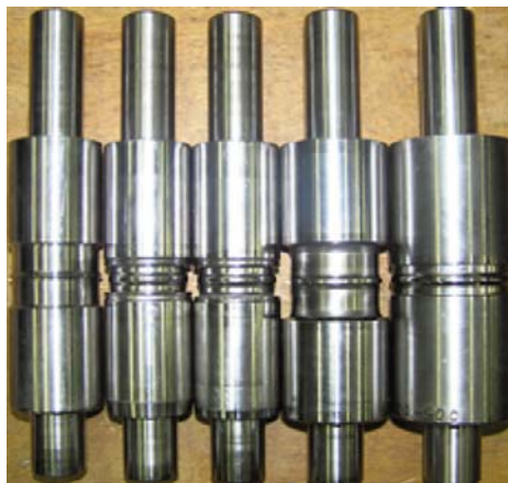
Fig. 6 Thorns on rolling bearing rings
