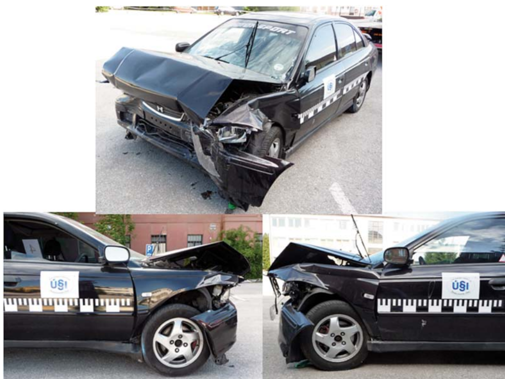
Fig. 7 Damage of the car Honda Accord (EES = 58 km/h)
