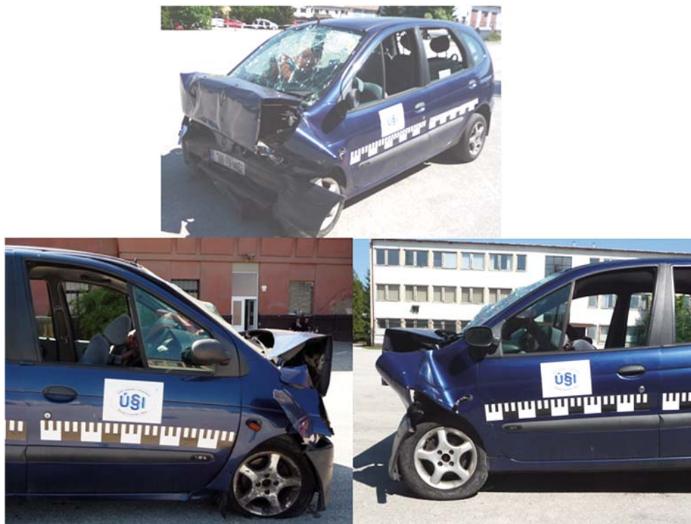
Fig. 6 Damage of the car Renault Megane Scenic (EES = 72 km/h)
