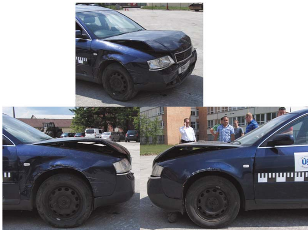
Fig. 8 Damage of the car Audi (EES = 18 km/h)
