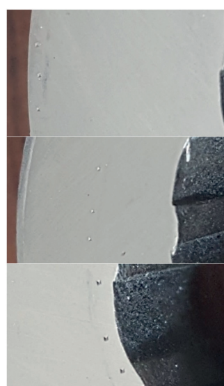
Fig. 2 Hardness measurements - sample and places
