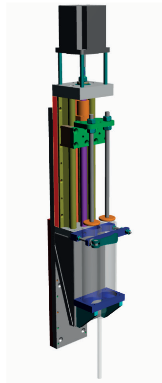
Figure 3 3D model of paste extrusion module
