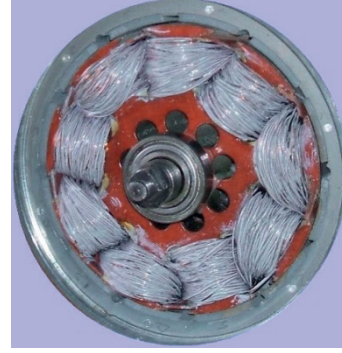
Figure 9 Photograph of prototype SMPM without bearing plate [8]
