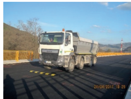
Figure 13 Dynamic load test of the Zvolen-Pstrusa highway bridge subjected to the heavy truck F_v = 320 \text{ kN} passing over the standard irregularity
