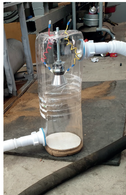
Figure 3 Experimental setup for ultrasound purification and utilization of ICE exhaust gases
