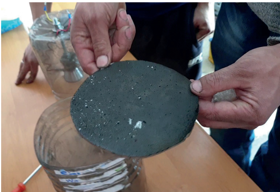
Figure 5 Ultrasonic wave reflector after operation of the experimental setup
