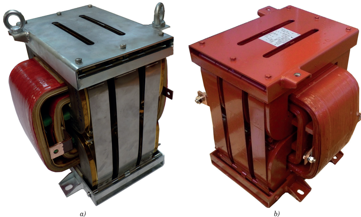
Figure 4 Photography of isolation transformer T10-200-2000/893: a) a prototype of the transformer with a built core made from AMM; b) a new design with a bent core made of 0.1mm thick transformer sheet
