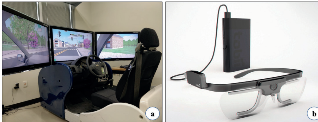
Figure 1 Morgan State University's driving simulator (a) and Tobii Pro Glasses2 eye-tracking system (b)
