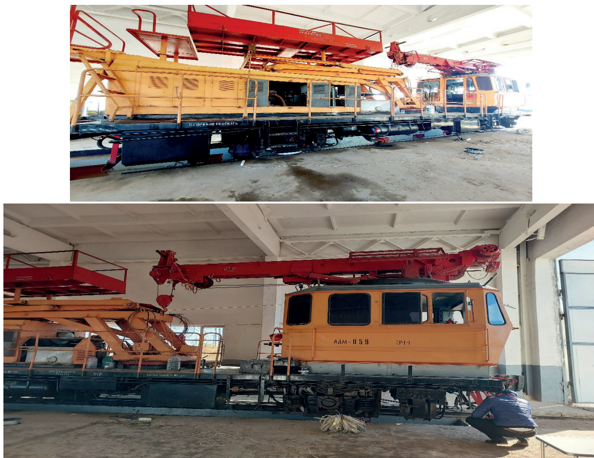
Figure 1 Photos of an ADM type rail service car
