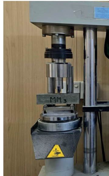
Figure 7 Flexural strength testing
