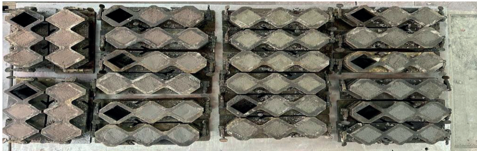
Figure 4 The casted specimens
