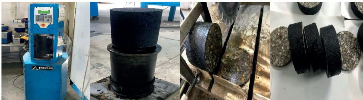
Figure 12 IDT preparation and cutting
