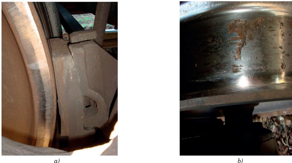
**Figure 1** The elements of the brake pad/wheel tribotechnical assembly that are inoperable due to the BLT design features;
