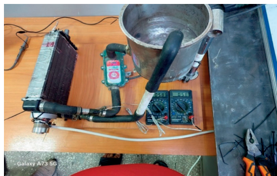
Figure 2 Experimental bench for cleaning radiator tubes
