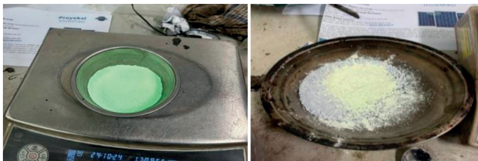
Figure 1 Thermoplastic road marking paint and phosphorus powder
