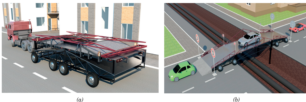
Figure 2 Municipal modular mobile overpass: a) transport position with folded modules; b) operational position over a trench
