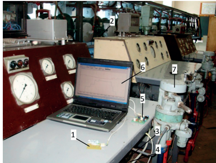
Figure 3 The diagnostic system for the brakes of a passenger car in the testing laboratory: 1 - light indication of a car; 2 - brake cylinder sensor; 3 - brake line sensor; 4 - electro-pneumatic brake sensor; 5 - microcontroller; 6 - laptop with software; 7 - driver's lever
